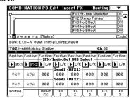
In the following example, the "Chain" box between IFX1 and IFX2 is checked so that the IFX1 output is sent to IFX2. "IFX1: 001: St. Amp Simulation" and "IFX2: 020: Stereo Flanger" are inserted to Timbre 1. "IFX2: 020: Stereo Flanger" is inserted to Timbre 2. The figure above ("Routing" pages) shows these settings. (In this example, IFX 3, 4, and 5 are not being used.)
